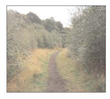
Where it is anticipated that horseriders will use part of a converted route, a segregated bridleway measuring a minimum of 2.0 m in width will be required. Such bridleways should be surfaced in grassed gravel. This surfacing is made up of a 150mm deep aggregate base course, covered in a 150mm deep mixture of aggregate and top soil and seeded in ryegrass.
