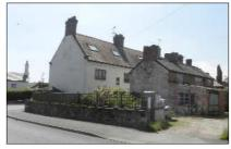
boundary wall fronting Wrexham Road and adjoining number 1 High Street has been repaired using a strong cement mortar in a ribbon course which detracts from its character and accentuates the decay of the original stonework.
